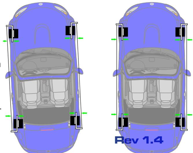
both sides by equal (but opposite) amounts until it is. The front-rear comparison is irrelevant, only the side-to-side matters. The picture on the left shows a bad thrust angle, the right shows a correct thrust angle. Double-check the toe once the thrust is set.
