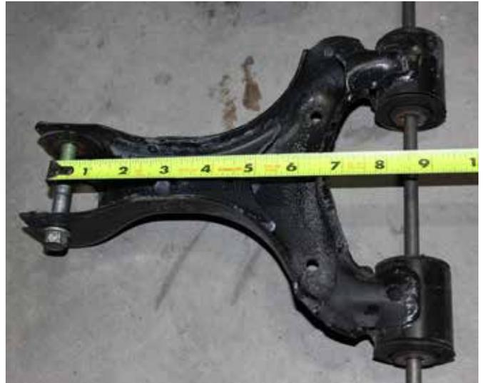
4. Install the arms. Be sure to use the included hardware on the outer bushing (the one that's installed in the upright), as the stock hardware is just barely too short. Leave the hardware loose for now.
