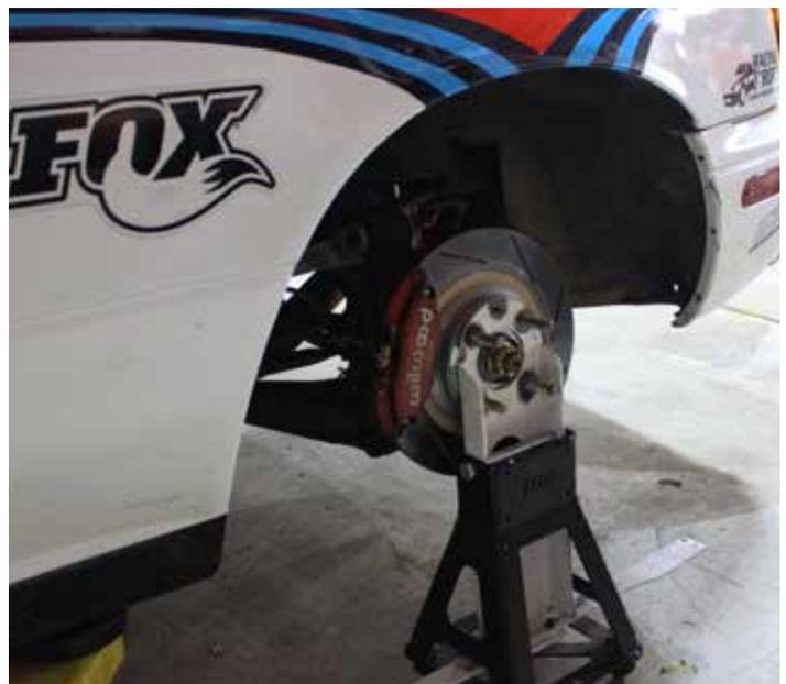
6. That's it, you're done with the installation! For future adjustments, take the wheels off and change the camber as desired (again, a half-turn =  $0.25^\circ$  of camber). Be sure to only tighten the bolt on the outer bushing fully with the suspension loaded. Be sure to tighten the jam nut on the control arm itself as well.
