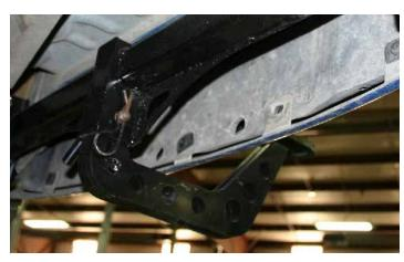
**Receiver Hitch Attachment only:** There is an additional hole at the top of the hitch (4) to eliminate the typical hitch wobble. You'll run the included bolt through the hole and tighten it down. You don't have to use this, but it is suggested. That's it, you're done. Now go tow something!
