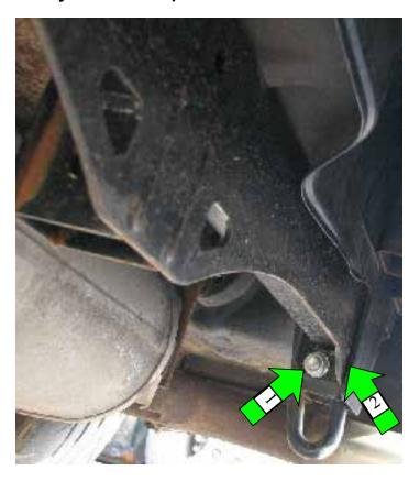
3. Press the hitch back into place. Slip all of the bolts through the holes before you tighten any of them. Use the "nutplates" for the upper bolts on both sides (3). Once all of the bolts are in place with nuts, tighten them all. Be sure to use a washer under the bolt head and the lower nut. The upper nut with the nutplate needs one under the bolt head but not under the nut.
