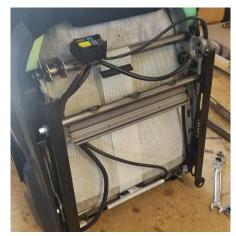
4. Hidden behind the recline adjustment handle there is a phillips head screw that needs to be removed. Next, at the front of the same plastic trim piece there is a plastic clip holding the trim to the seat frame. You can remove the clip with a pair of pliers or carefully flex the trim piece, sliding it off the plastic pin. The trim will still be attached to the seat, but you will be able to flex it out of the way to access a bolt in a later step.
