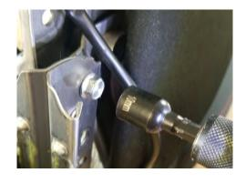
6. Next remove the fore/aft sliding adjustment handle from the seat. There is a small torsion spring attached to a pin where the handle pivots. Remove the spring with pliers and then remove the pin and the handle. You may need to temporarily remove the electric harness plug from its bracket to gain enough clearance to remove the pin.
