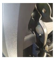
5. Using a 10mm wrench or socket, remove the two small bolts near the front of each seat rail.
