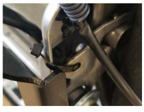
9. Locate the new pair of mounting rails for the left or right seat you are working with and position them at the inner and outer sides of the seat as labeled. Position the rear end of the new rails inside the flange at the rear of the seat, and outside of the threaded tube at the front end of the seat. You will reuse the 14mm bolts from the previous step to attach the new rails.
