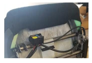
3. Now the seat can be removed from the car. This is easiest with the top down and with the seatback mostly upright. Prepare a clean, flat surface and place the seat on its back, allowing access to remove the factory seat rails.
