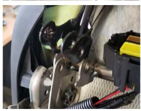
7. Now you will be able to remove the four 14mm bolts from the seat assembly and remove the factory seat rails. One of the bolts holds the seat belt receiver and will remain connected to it along with a small wiring harness you should be careful not to damage. As you remove the factory rails, there will be a steel tube at the rear of the seat that can fall away if the sliders are spread apart. Put this assembly and the seat rails aside. You will not reuse them.
