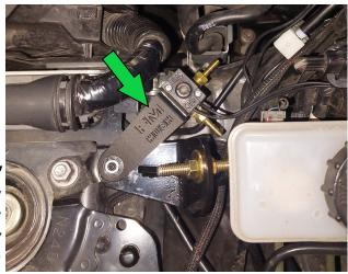
1. Loosely assemble pivoting foot onto bracket using 5/16<sup>"</sup> hex nut and pair of 5/16" flat washers as shown.
