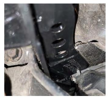
5. Holding the threaded foot in place against the master cylinder, turn the thinner jam nut with the ½" wrench until a little preload is applied between the bracket and the nose of the master cylinder. Do not go crazy here. A little bit of preload is plenty.
