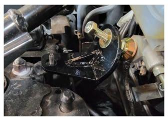
6. With the foot in place and pre-loaded to the master cylinder, spin the outer  $\frac{1}{2}$ " hex nut down until it becomes snug against its washer and bracket. Hold the foot still with the 5/8" wrench and snug down the outer  $\frac{1}{2}$ " nut to lock things in place. DO NOT OVER-TIGHTEN.
