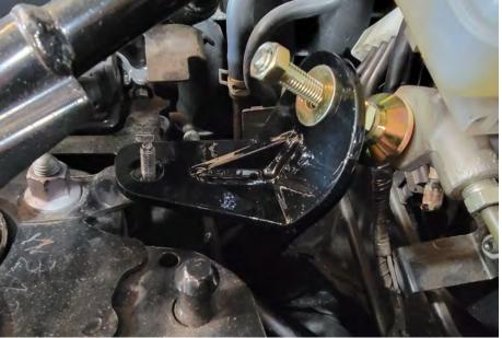
2. Lower assembly into place, over the upper stud and onto the lower stud at the same time. The bracket should be positioned flat against the frame rail surfaces.
